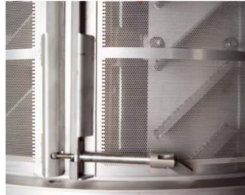
Perforated Screen used for most dryer applications
