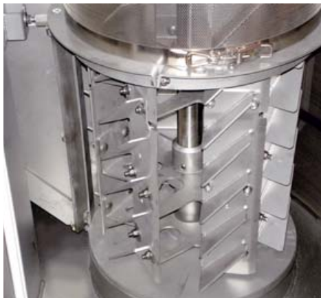
Rotor area of a 2016 BF Dryer
