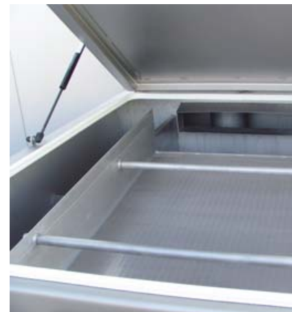
Tempered water system tank with integrated fines removal screen system to remove down to 300 µm particles
