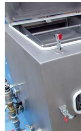
Tempered water system tank with integrated fines removal screen system to remove down to 300 µm particles
