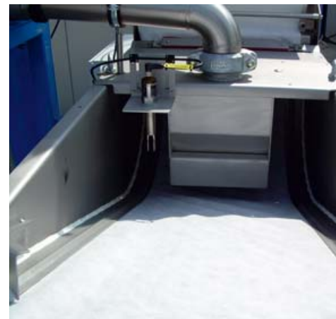
Tempered water system tank with band filter medium to remove down to 20 µm particles
