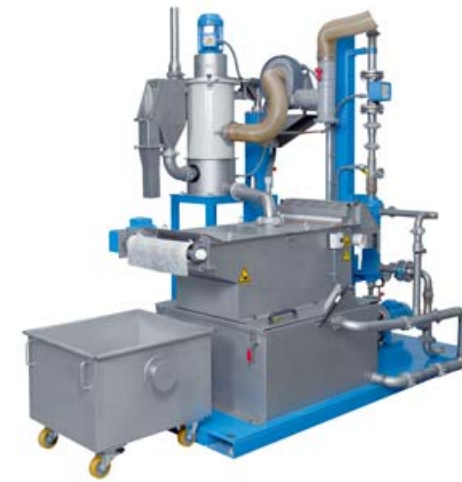
MB 500-BF2 with band filter in tank
