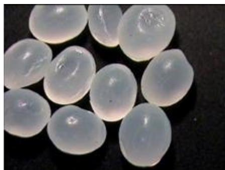
Fig. 5 Crystalline PLA pellets
