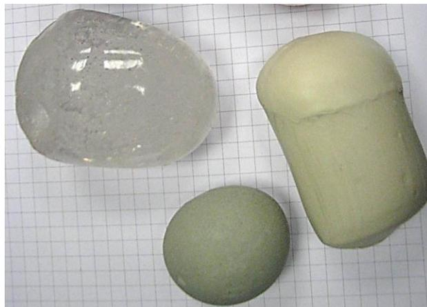
Fig. 7 Start-up material downstream of the MCD
